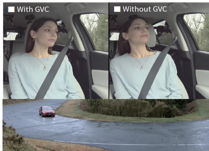
* In-house passenger seat comparison of left-hand turn at 30 km/h (lateral acceleration of 0.4 G)
